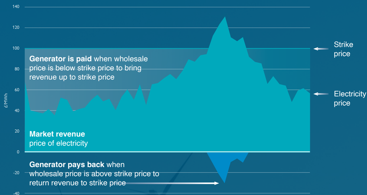
Figure 1-6: Diagram of CfD operation: the mechanism for delivering a fixed price in variable wholesale market. Source: House of Commons Library.
